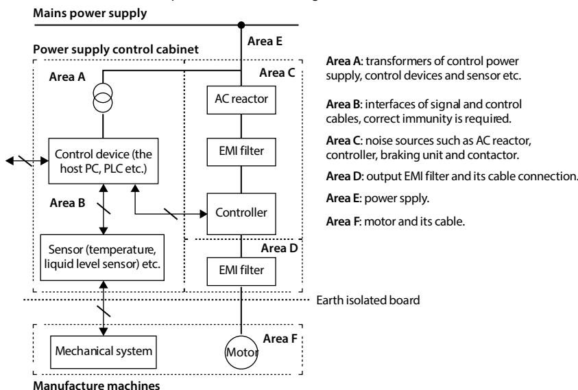
Figure 4-25 System wiring
