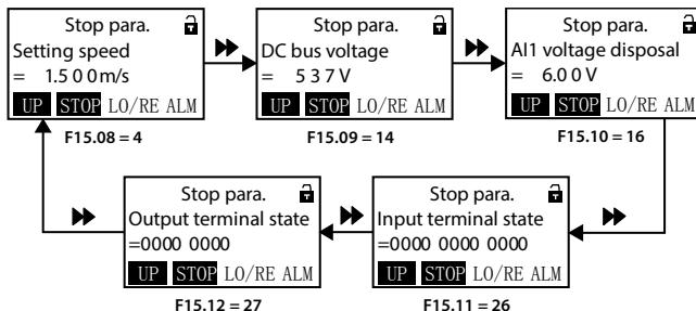
Figure 5-6 Switching display parameters at stop status
