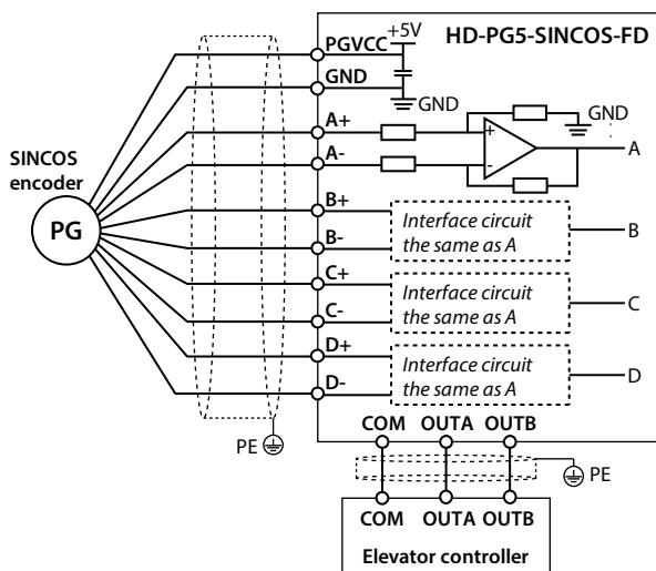
Figure 4-21 Connection of SINCOS encoder
