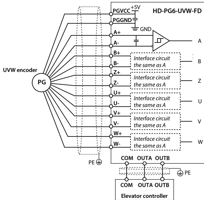
Figure 4-23 Connection of UVW encoder
