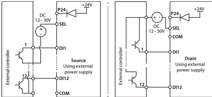
Figure 4-8 Source / Drain connection when using external power
