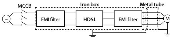
Figure 4-30 Reducing RF interference
