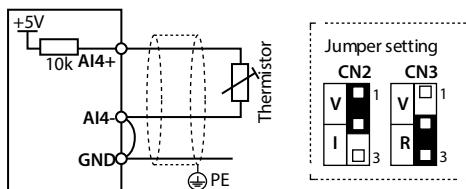
Figure 4-13 AI4 connection (AI4 = overheat detection signal input)
