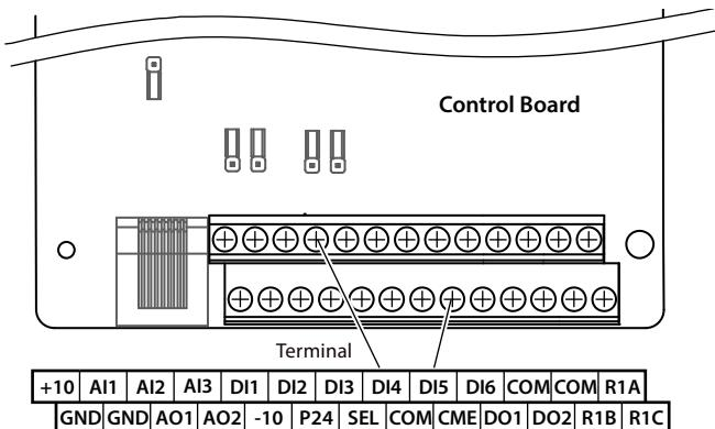
Figure 4-3 Control board terminal
