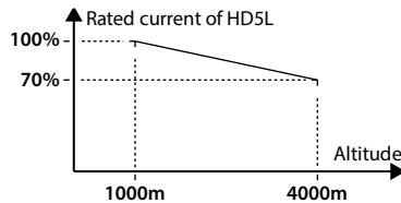
Figure 1-1 Derating curve of rated current and altitude
