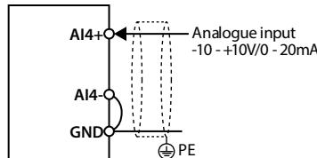
Figure 4-12 AI4 connection (AI4 = analogue input terminal)
