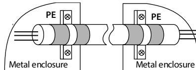
Figure 4-27 Shielded cable connection
