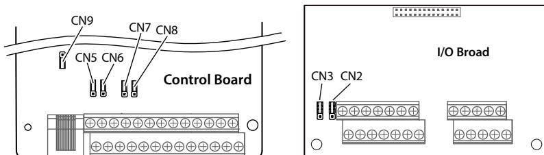
Figure 4-5 Jumper position
