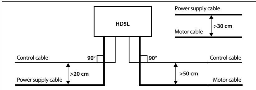
Figure 4-26 System wiring
