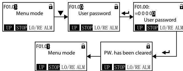
Figure 5-9 Operation of clearing user's password
