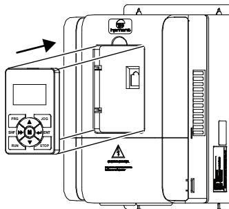
Figure 3-2 Install keypad
